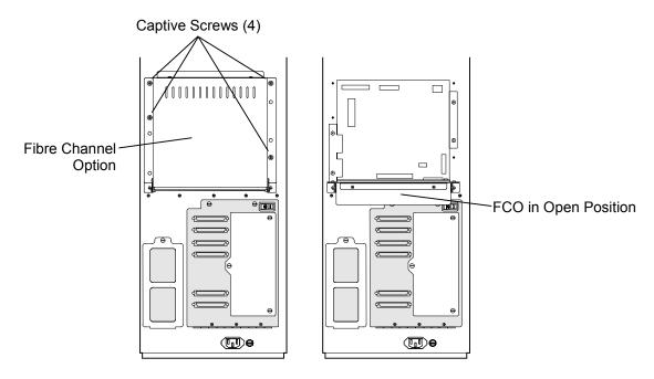
Figure 9-2 Fibre Channel Option in Closed and Open Positions (Type A Shown)
